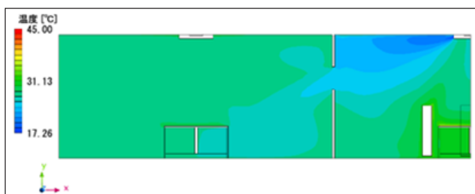
Figure 13. Air temperature of Case 3. The target zone's average air temperature was 27.4^\circ\text{C} , while the average air temperature in the non-target zones was 27.6^\circ\text{C} , respectively
