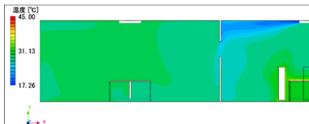
Figure 19. Air temperature of Case 6. The target zone's average air temperature was 27.2°C, while the average air temperature in the non-target zones was 28.2°C, respectively
